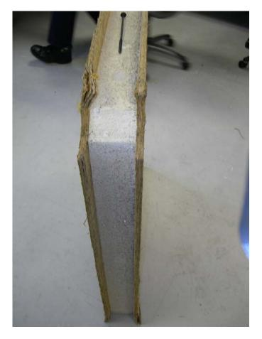
Please look at this picture. What you are seeing is the wall assemblies that are currently being put up in the Laurel Hill subdivision in Lorton. This wall assembly is prefabricated and is made up of 2 pieces of OSB with Styro-foam insulation between them. There are occasional 2x4's "Studs" in them with additional 2x4's as the sills and headers. If someone tries to get out from the inside it will be very difficult. Also the insulation and sound deadening is impressive. Hotter fires quicker!
